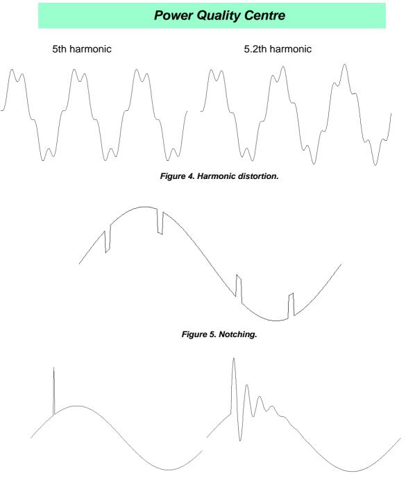
Figure 6. Typical transients from lightning (left) and system switching (right).
